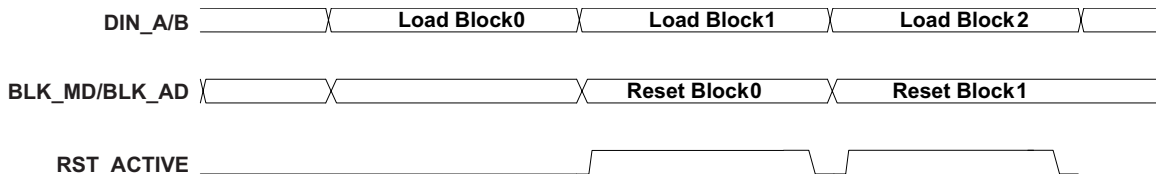
Figure 12. Typical Phased Mirror Clocking Pulse Sequence
