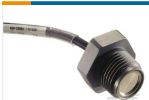
TE Part #LM31-00000F-005PG 5PSIG LIQUID LEVEL PRESSURE TRANSDUCER
