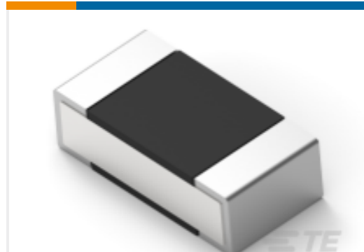
TE Part #7-2176305-0 RP 1E 0.1W 562R 0.1% 25PPM 5K RL
