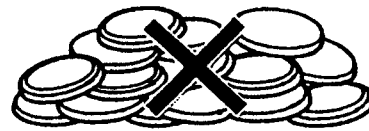
Example of stacked and jumbled batteries
