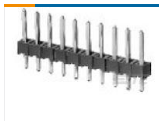
TE Part #5-146280-6 06 MODII HDR SRST B/A .100CL
