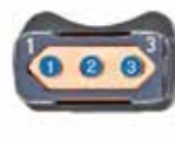
Using Socket (Female) Contacts
