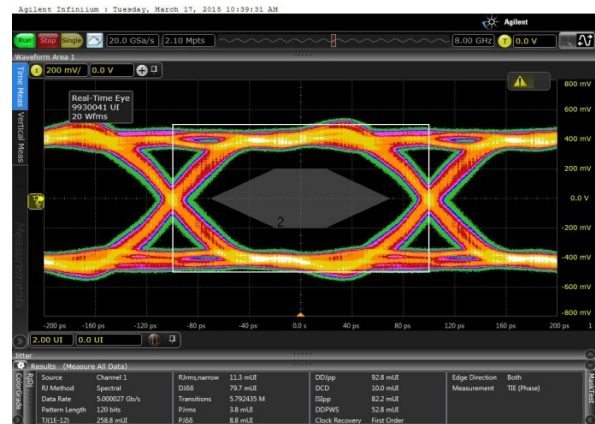
Figure 35. Eye at 5-Gbps Bit Rate with Increased Output Swing
