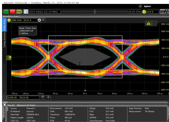
Figure 34. Eye at 5-Gbps Bit Rate with Default Output Swing
