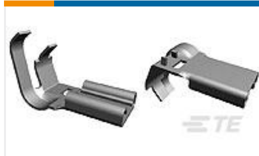
TE Part # 150699-2 187 FASTON,FLAG,REC.,20-16 AWG, TPBR
