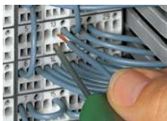
CAGE CLAMP® connection Inserting a conductor via 210-719 Operating Tool (2.5 x 0.4 mm blade).
