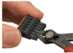
Coding a female connector by removing coding finger(s). (MCS MINI SL)
