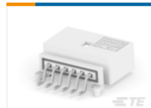
TE Part # 2317023-2 6pos MQS .63 header 90deg SMD
