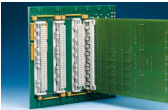
Coding Strip FL mounted on a backplane.
