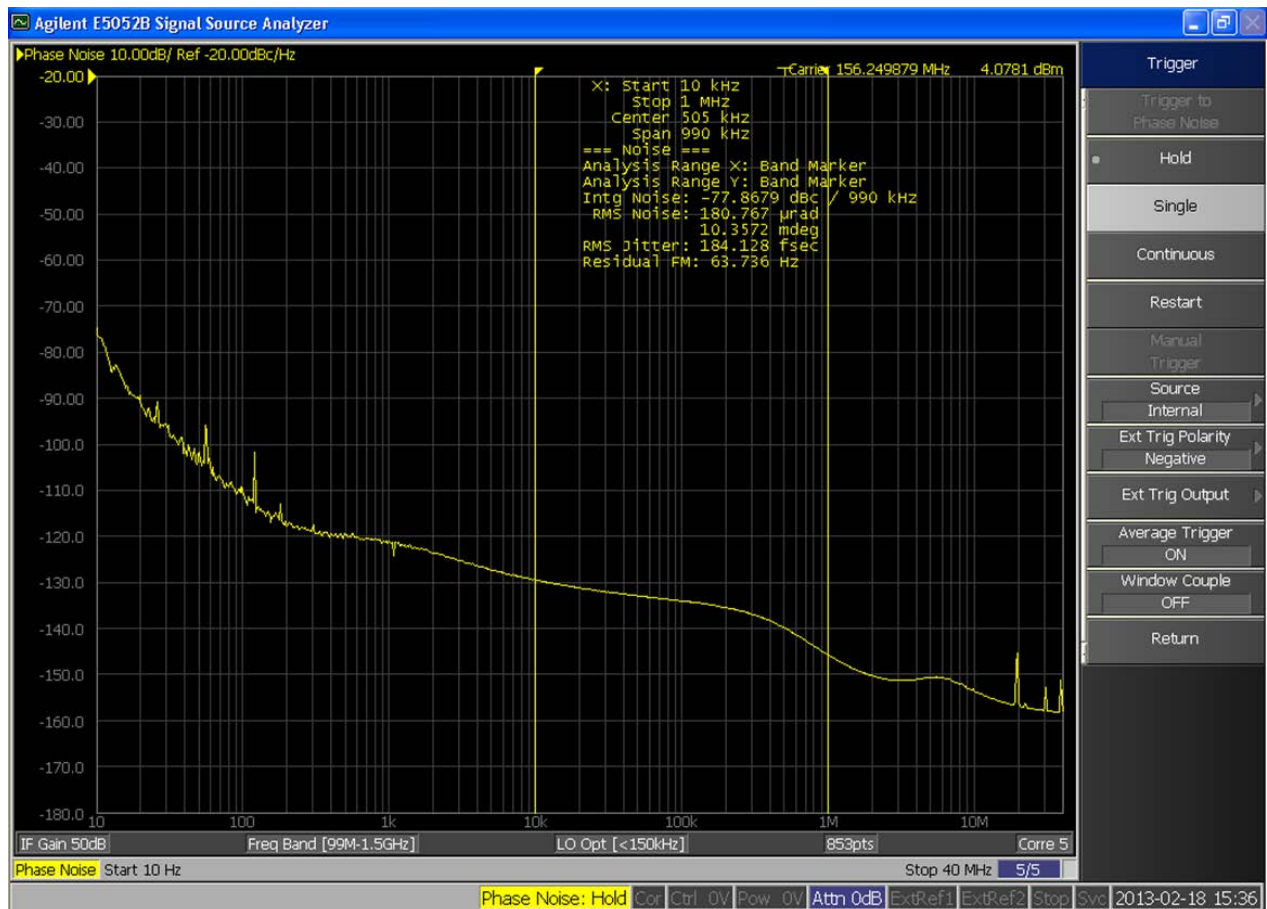
Figure 1. Si535/536 Typical Phase Noise at 156.25 MHz
