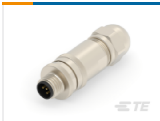
TE Part #T4111412051-000 M12 M, 5P GOLD B_CODE S SHIELDED PG9
