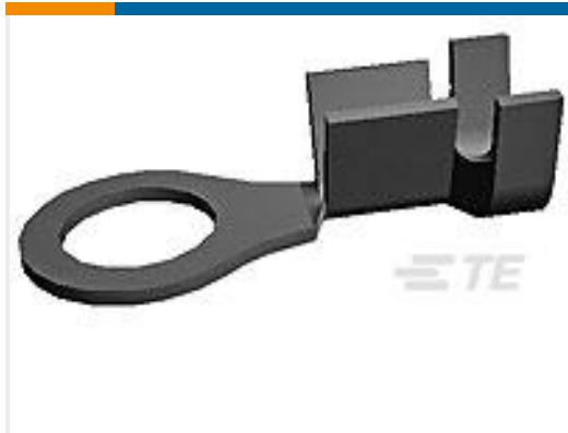
TE Part #42037-1 RING TERMINAL 22-18 AWG TPBR
