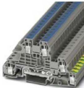
Installation ground terminal block, Screw connection, cross section: 0.2 mm 2 - 10 mm 2 , AWG: 24 - 8, width: 8.2 mm, color: gray, mounting type: NS 35/7,5, NS 35/15
