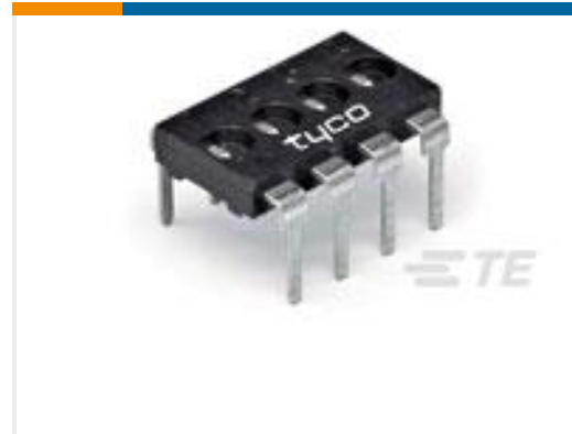
TE Part #1825190-7 DIP Shunt,8 pos
