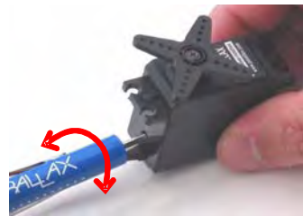
Gently turn screwdriver to adjust potentiometer
