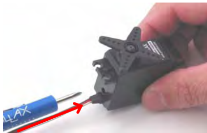
Insert tip of Phillips screwdriver into potentiometer access hole.
