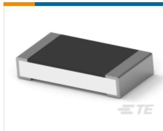
TE Part #4-2176391-7 RQ 1206 37K4 0.1% 10PPM 5K RL
