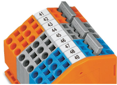
4-conductor through terminal blocks, angled type, formation of groups with 3-way, comb-style jumper bars
