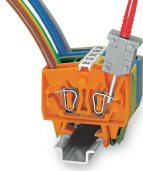
Testing via CAGE CLAMP® on the current bar (max. nominal current: 6 A). CAGE CLAMP® clamps individual test contacts. The maximum test voltage is 400 V.
