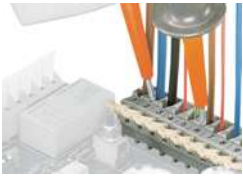
Testing with test probes.
