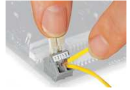
Inserting/removing a conductor via finger-operated lever – 256 Series.
