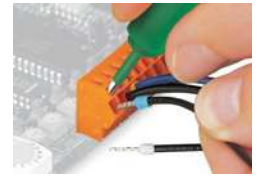
Inserting/removing a ferruled conductor.
