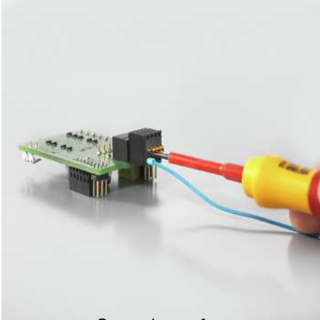
Operating safety Through PUSH IN connection system
