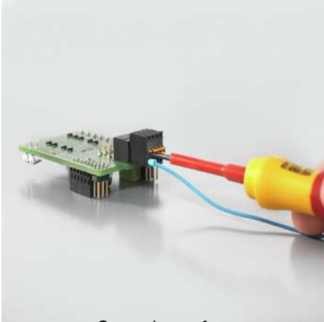
Operating safety Through PUSH IN connection system
