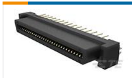
TE Part #1734101-3 Champ050 series, 30pos, Au over PdNi
