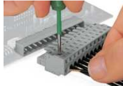
Inserting a conductor via 3.5 mm screwdriver – CAGE CLAMP® actuation perpendicular to conductor entry.
