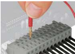
Testing – female connector with CAGE CLAMP® Integrated test ports for testing perpendicular to conductor entry via 2 or 2.3 mm Ø test plug
