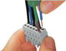
Inserting a conductor via 3.5 mm screwdriver – CAGE CLAMP® actuation parallel to conductor entry.
