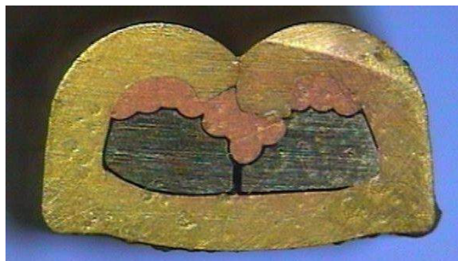
3. Terminal and wire are bonded at the atomic level and adhesion occurs
