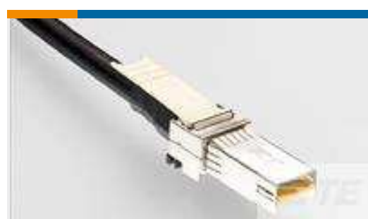
TE Part # CAT-Q17-N490333 QSFP56-Four SFP56 Cable Assembly: 26 AWG
