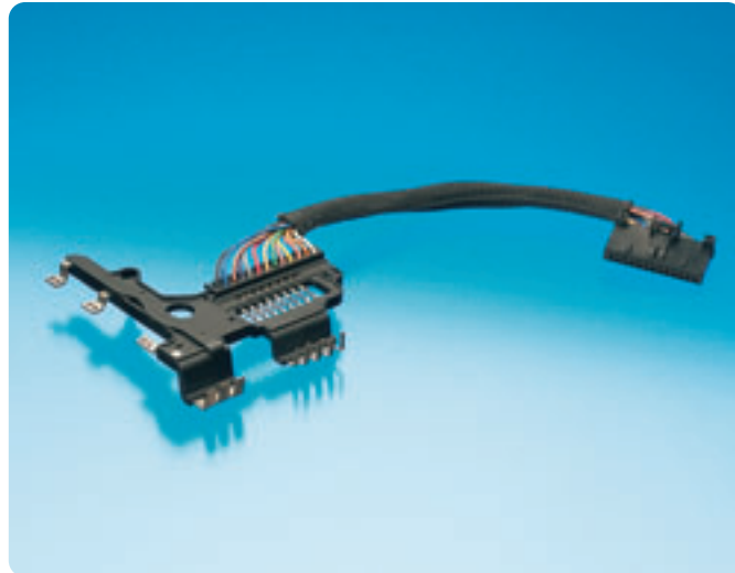
Steering EPAS (Electrical Power Assistance Steering)
