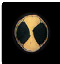
Press-fit geometry cross section (bow-tie)
