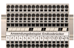
Continuous jumpers (2002 Series) readily connect an endless number of terminal blocks to each other via single jumper slot. Use the second jumper slot for additional commoning or testing.
