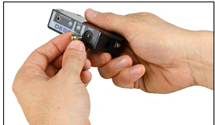
Figure 10. Changing the park snap on the 19652 Multi-Mount Monitor
