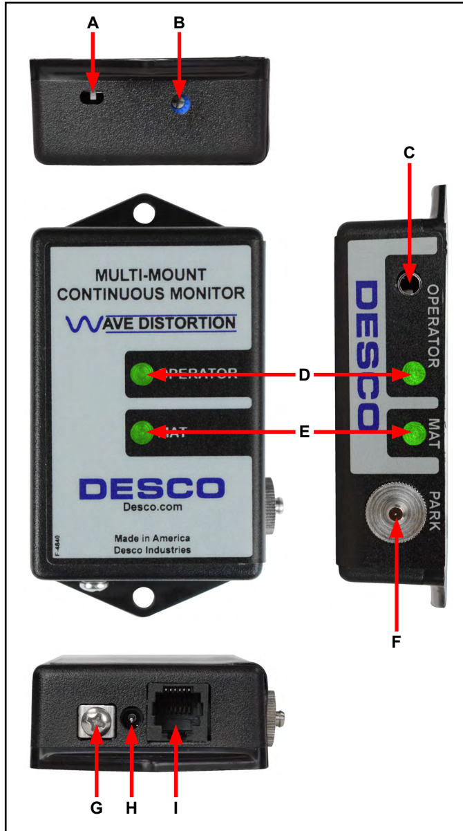
Figure 5. Multi-Mount Monitor features and components
