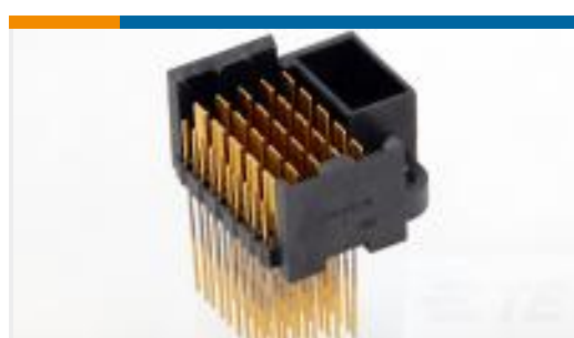
TE Part #5120737-1 HS3 B/P HDR ASY 6R 60 P LEV 1
