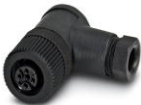
Connector, 4-position, Socket angled M12, A-coded, Screw connection, Knurl material: Plastic, Cable gland Pg7, External cable diameter 4 mm ... 6 mm
