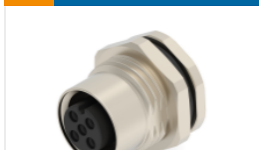
TE Part #T4131012051-000 M12,REAR MOUNT,FEMALE,A,5P, SOLDER WIRE
