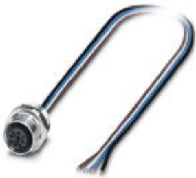
Sensor/actuator flush-type socket, 4-pos., M12, A-coded, front/screw mounting with Pg9 thread, with 0.5 m TPE litz wire, 4 x 0.34 mm 2 , stainless steel version
