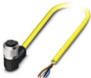
Sensor/actuator cable, 4-position, PVC, yellow, free cable end, on Socket angled M12 SPEEDCON, A-coded, cable length: 15 m
