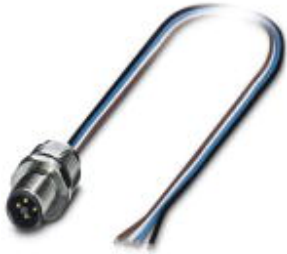
Flush-type connector, Power, 4-position, Plug, M12, T power, Front mounting, M16 x 1.5, Individual wires, cable length: 0.5 m
