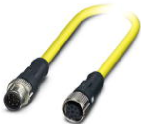
Sensor/actuator cable, 8-position, PVC, yellow, Plug straight M12 SPEEDCON, A-coded, on Socket straight M12 SPEEDCON, A-coded, cable length: 20 m
