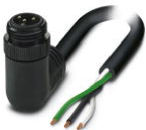
Power cable, 3-position, PVC, black, Plug angled 7/8"-16UNF, A - standard, on free cable end, A - standard, cable length: 10 m
