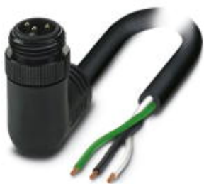
Power cable, 3-position, PVC, black, Plug angled 7/8"-16UNF, A - standard, on free cable end, A - standard, cable length: 5 m
