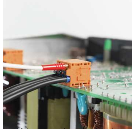
Maintenance through test point
