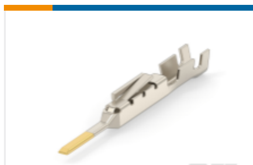
TE Part #1318110-1 Contact: Component To Wire ; 5A, 28-18 wire size, gold plated
