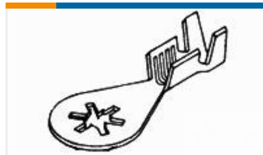
TE Part #61795-3 RING 18-14 AWG TPBR
