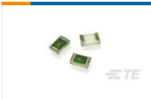
TE Part #2176092-2 RP 2A 0.25W 665R 0.1% 25PPM 1K RL
