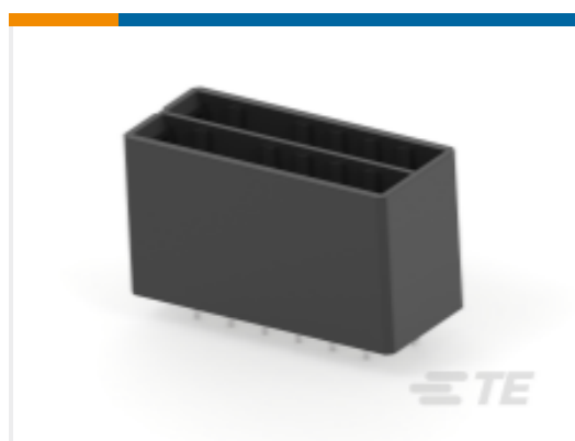
TE Part #1-917337-3 Header Assembly: Wire-to-Board, 15A, gold or tin plated
