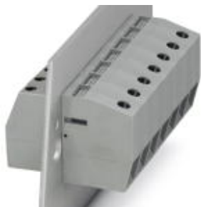
Panel feed-through terminal block, connection method: Screw connection, Screw connection, number of positions: 1, cross section: 6 mm 2 - 35 mm 2 , AWG 10 - 2, color: gray
